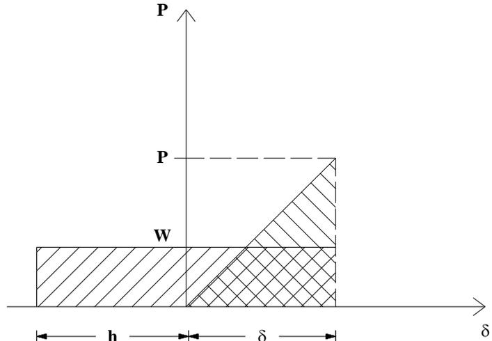
$$\begin{aligned} \text{Siendo: } \delta &= \frac{P \times L}{\Omega \times E} \rightarrow P = \frac{\Omega \times E}{L} \times \delta \\ &\Rightarrow W(h + \delta) = \frac{\Omega \times E}{2L} \times \delta^2 \\ &\Rightarrow -\frac{\Omega \times E}{2L} \times \delta^2 + W \times \delta + W \times h = 0 \end{aligned}$$
