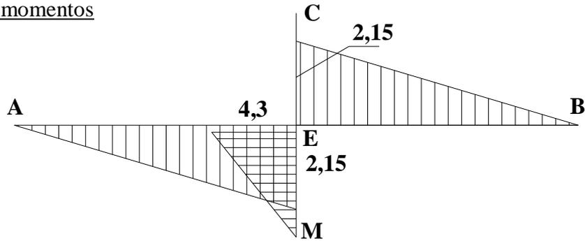
$$M_E^A = M_E^B = 3,75 \times F = 3,75 \text{ cm} \times 0,5734 \text{ tn} = 2,15 \text{ tncm}$$
