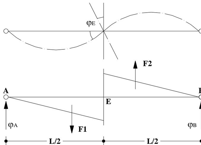
$$F_1 = F_2 = \frac{3,75 \times F (\text{cm}) \times 15 \text{ cm}}{2 E \times I} = \frac{28,125 F}{E \times I} \text{ cm}^2$$
